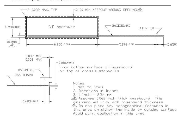
Figure 4: Chassis I/O Aperture Requirements (rear and side view—see Figure 3 for datum location)
