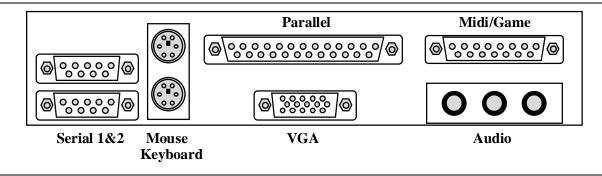
Figure 6: Example Multimedia I/O Back Panel
