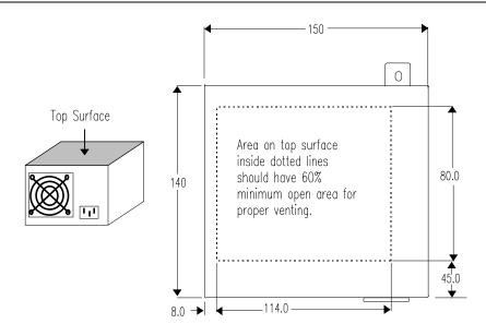
Figure 17: ATX Power Supply Suggested Venting (all dimensions in millimeters)
