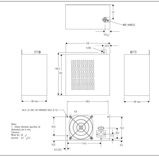
Figure 9: ATX Power Supply Mechanical Diagram (all dimensions in millimeters)
