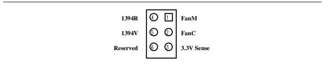
Figure 13: Optional Power Supply Connector Configuration
