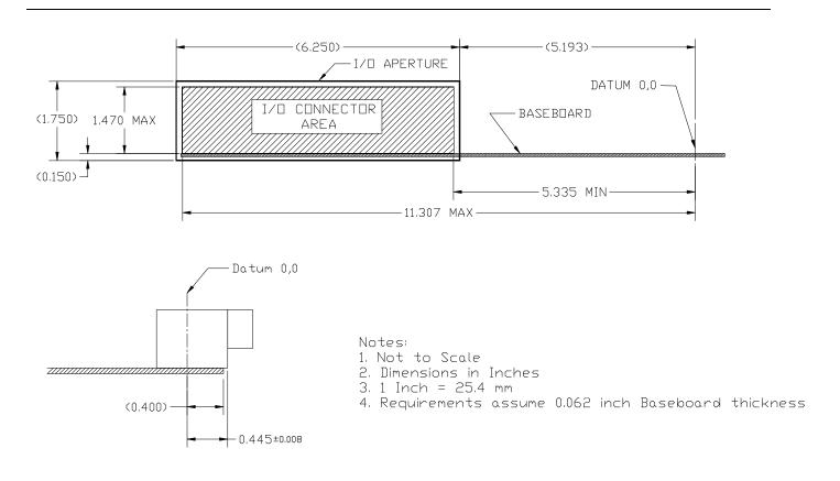
Figure 5: Baseboard I/O Connector Location Recommendation (rear and side view—see Figure 3 for datum location)
