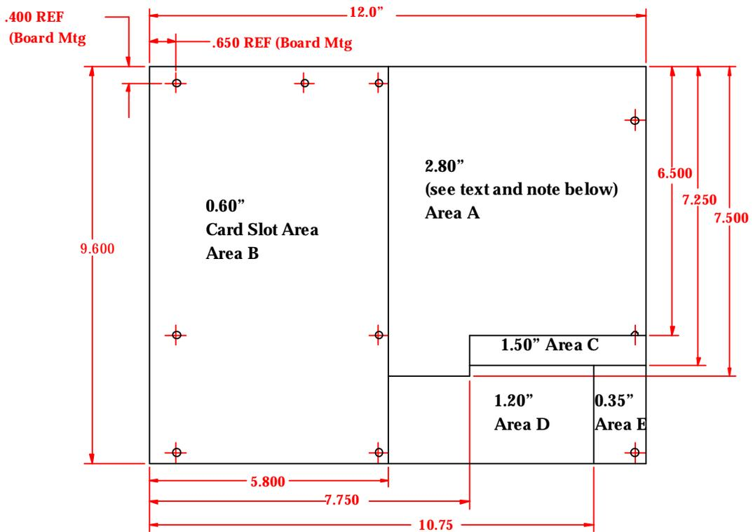
**Figure 8: ATX Motherboard Maximum Component Height Restrictions**
