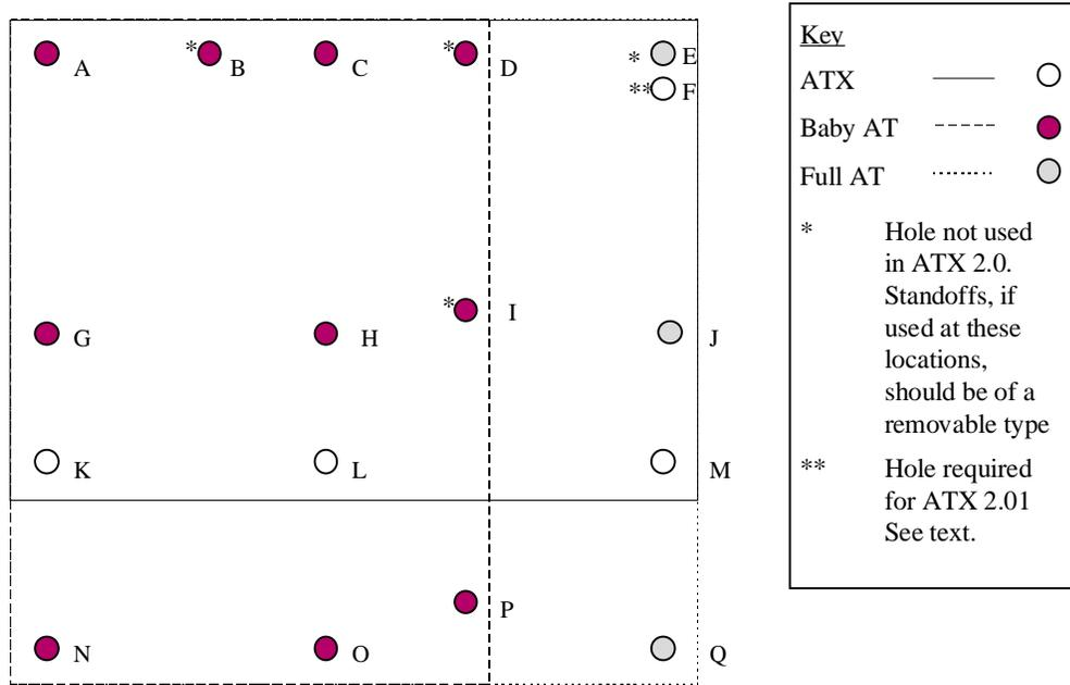
See the mechanical drawing in this specification for details on mounting locations and board sizes
