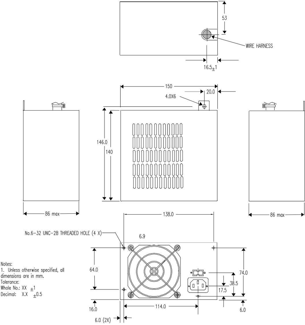
**Figure 9: ATX Power Supply Mechanical Diagram**
