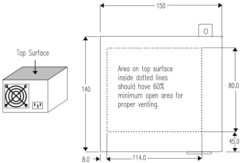
**Figure 17: ATX Power Supply Suggested Venting**
