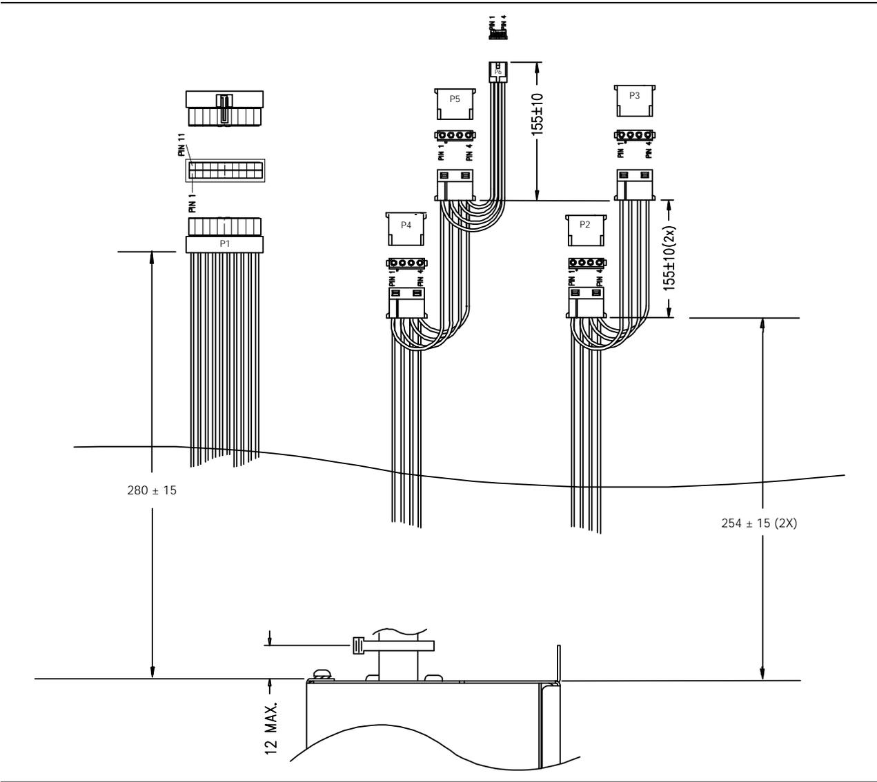
**Figure 16: ATX Power Supply Wiring Harness**
