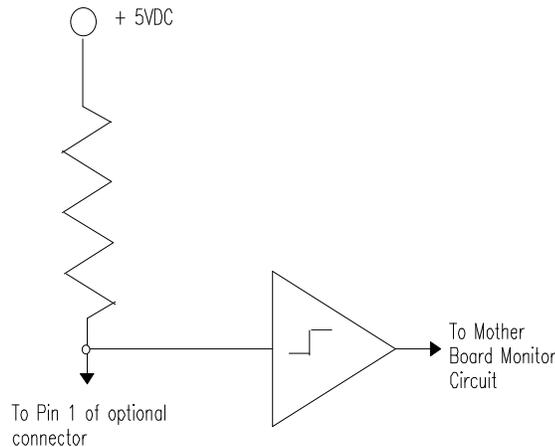
**Figure 14: Simple Implementation of a Fan Monitor Circuit**
